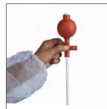
4. Blow out the pipette by pressing as the drawing indicates (point C).
