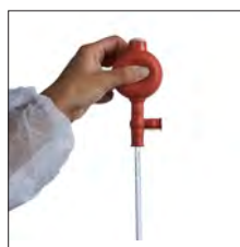
1. Evacuate the air by pressing the bulb, as the drawing indicates.
