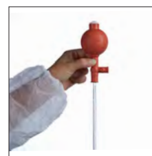
2. Intake by pressing on point B (↑)
