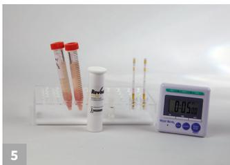
5 Place a new Reveal<sup>®</sup> test strip with the sample end down into the sample cup and set a timer for 5 minutes. Ensure the test strip comes into contact with liquid and begins to wick.
