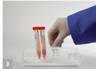
3 Re-cap the sample vial and mix by shaking for 10 seconds.
