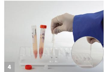
4 Using a 100  $\mu$ L fixed volume pipette, transfer 100  $\mu$ L of the sample extract from the sample vial into a new clear sample cup.
