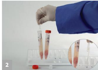
2 Remove the cap from the sample vial. Using a 200  $\mu$ L fixed volume pipette, transfer 200  $\mu$ L of the sample supernatant into the sample vial.
